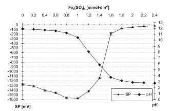
Fig. 4. Changes in the streaming potential (SP) and pH of a model HA solution, depending on the dose of iron(III) sulfate.
