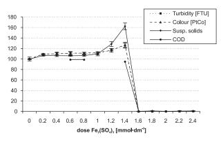
Fig. 2. Changes in the values of pollution indicators for an HA solution, depending on the dose of iron(III) sulfate, expressed as a percentage in relation to the initial model HA solution.
