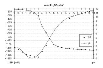
Fig. 5. Changes in the pH and streaming potential (SP) of a model HA solution during acidification with sulfuric acid.
