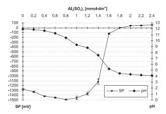
Fig. 3. Changes in the streaming potential and pH of a model HA solution, depending on the dose of aluminum sulfate.
